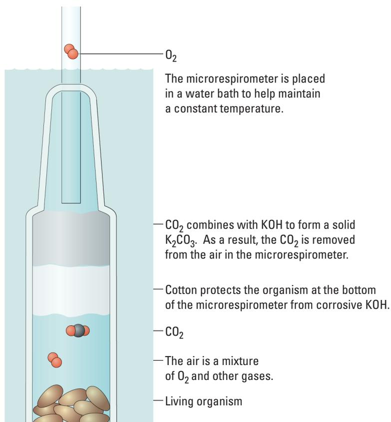
**Figure 1. Microrespirometer**
